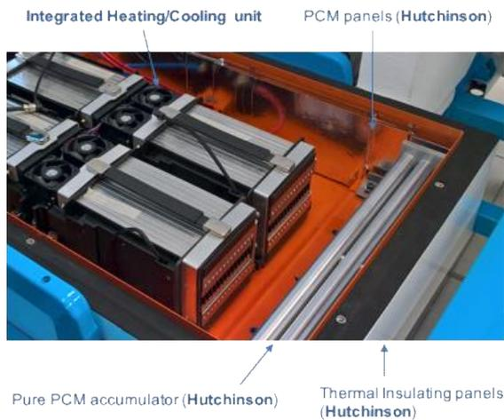
Fig.6: View of the battery pack enclosure.
