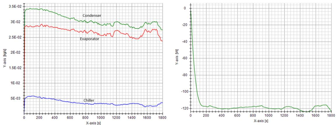
Fig.5: A: Refrigerant mass flow rate of the heat exchangers. B: Thermal power transferred to the food storage compartment.
