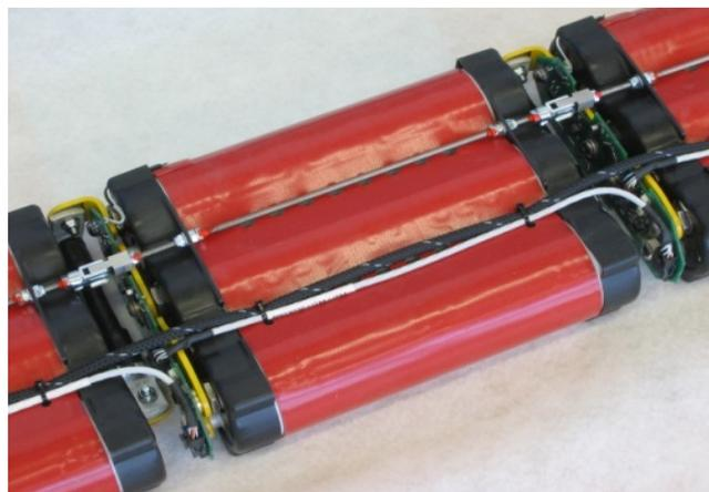
Fig. 4. Battery modules consisting of three battery cells connected in series. The battery monitoring electronics is located between two modules.
