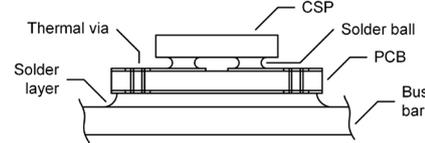
Fig. 7. Cross section of the CSP mounted on a PCB using the battery busbar for improved heat dissipation
