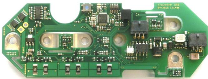
Fig. 3. Battery monitoring electronics showing the busbars directly soldered on the printed circuit board.
