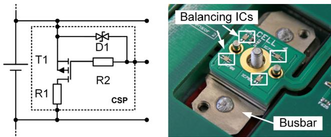
Fig. 6. Left: Equivalent circuit of the balancing IC; Right: chip-size-package (CSP) balancing MOSFET components mounted on PCB. For improved heat dissipation the PCB is soldered to the busbar below.
