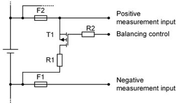
Fig. 5. Passive balancing circuit for a battery cell as part of a series connection of battery cells.
