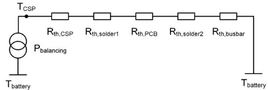
Fig. 8. Thermal equivalent circuit for a worst case estimation of the CSP temperature ( $T_{\text{CSP}}$ ) during balancing.
