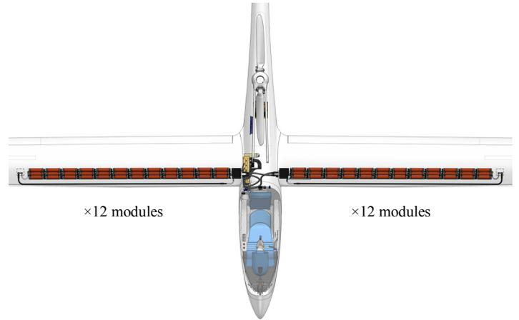
Fig. 1. Global overview of the Antares 20E glider from Lange Aviation GmbH showing its electrical powertrain.
