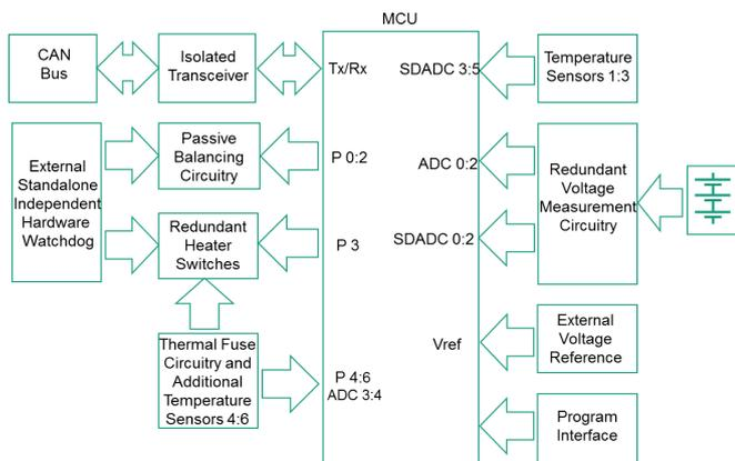
Fig. 2. Block diagram of the battery monitoring electronic circuit sensing the battery cell voltages and temperatures, performing passive cell balancing, and sending the collected data to a central computing unit (CCU) over a galvanically isolated CAN bus.
